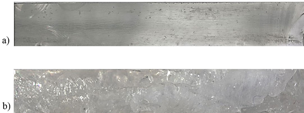
Figure 17. Macro photography of the fracture of the specimens PMMA (a) and PC (b)
